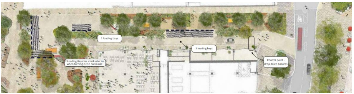
Image above: proposed layout to show loading bays bollard vehicle and pedestrian routes.
