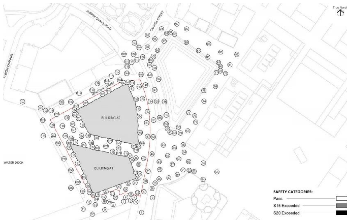
Image above: Configuration 3: Proposed Development with cumulative surrounding buildings, proposed landscaping and mitigation measures, ground level, annual safety.
