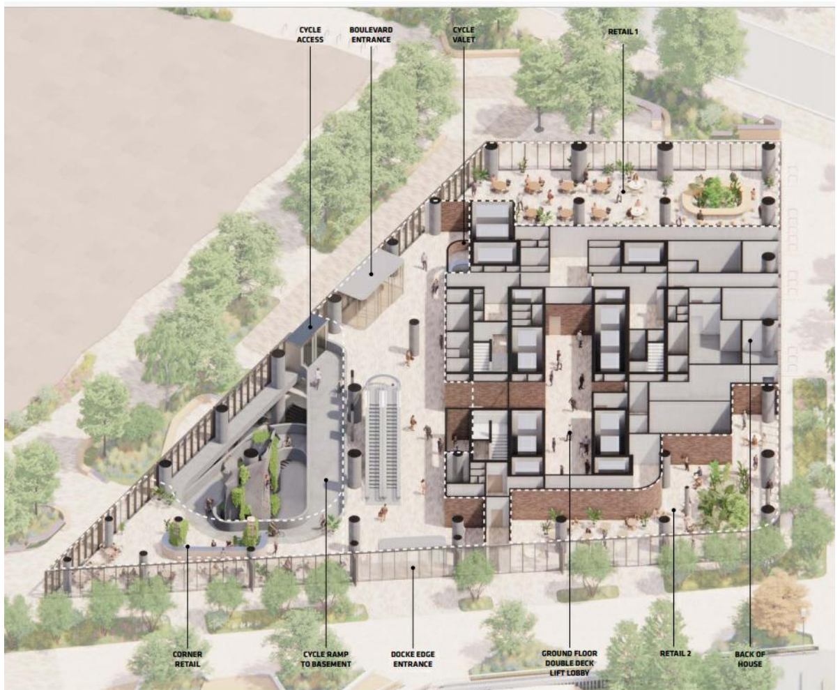
Image above: Proposed ground floor layout for Building A1 showing access points and layout of spaces
