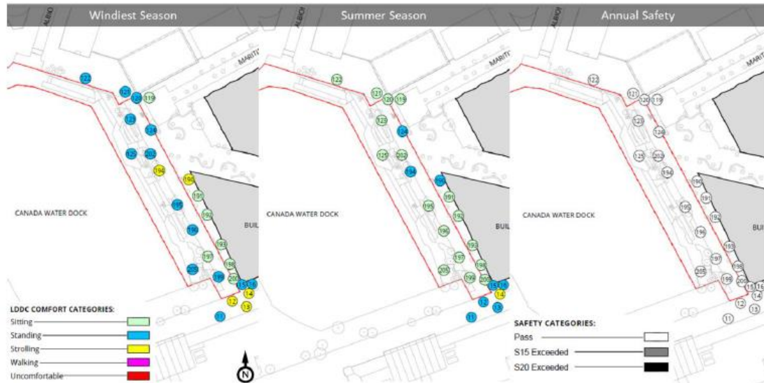
Image above: Configuration 4 (Proposed development with existing surrounding buildings and updated proposed landscaping) wind results
